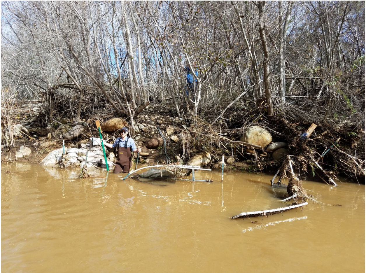
Figure 9. Picture of bent t-posts, dangling truck rope and antenna wire, broken debris panels (for DIDSON), and upended tuner box t-posts after the January 19, 2017 storm event. T-posts held by Samuel Bankston (Fisheries Biologist, PSMFC).
