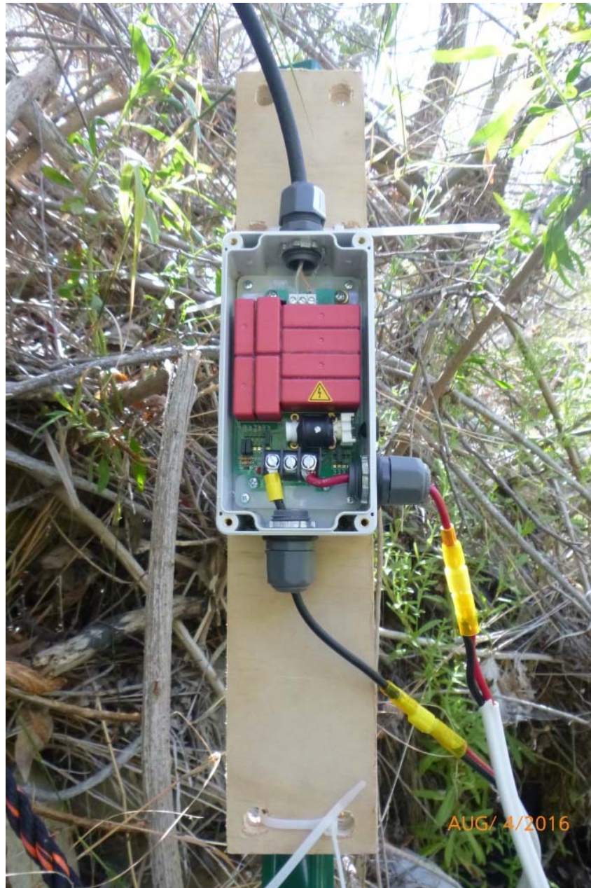
Figure 6. Picture of a tuner box screwed onto a wooden board mounted on a t-post at the Ventura River mainstem PIT tag array site.
