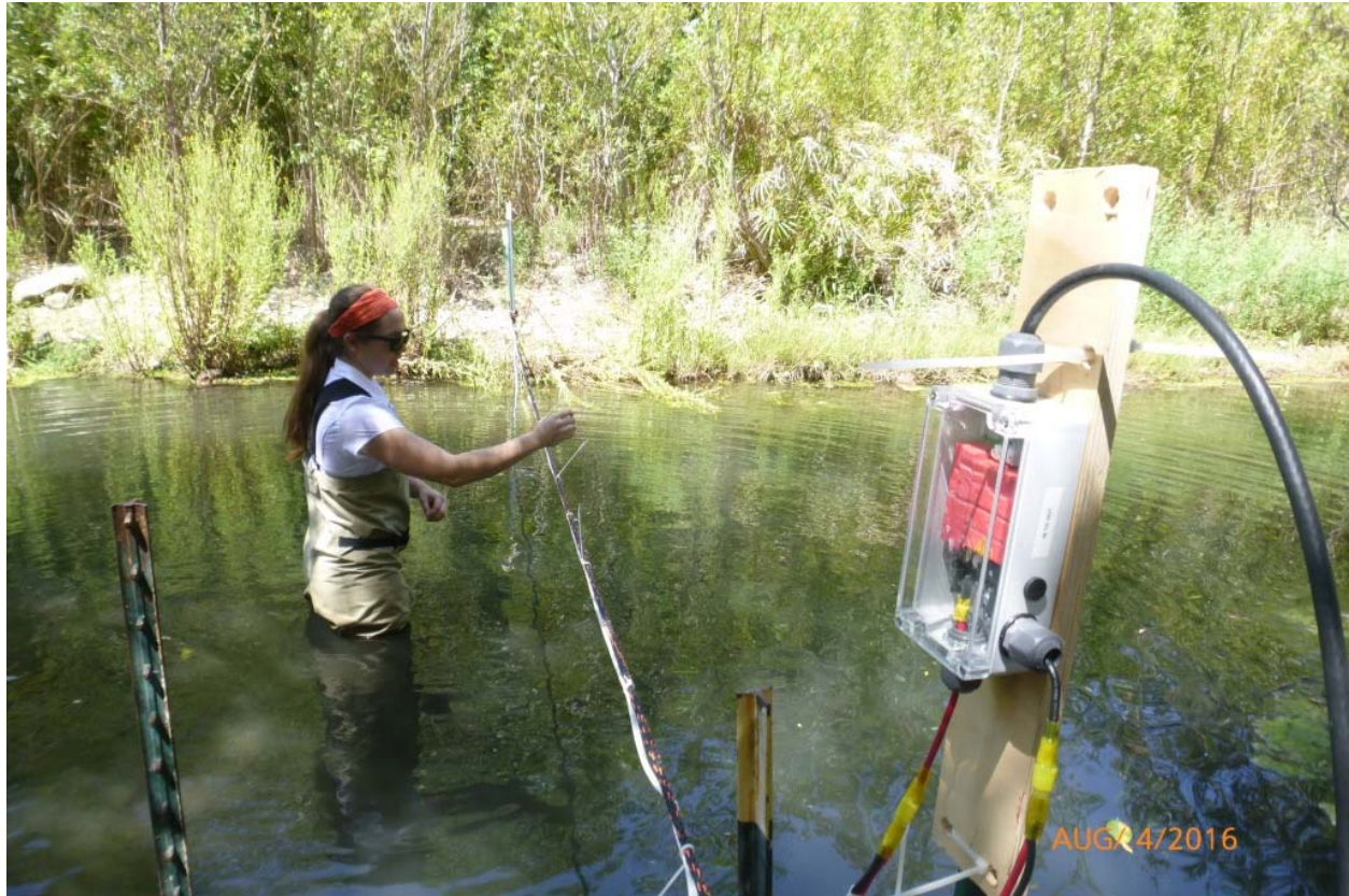
Figure 8. Picture of Kathryn Carmody (Fisheries Technician, PSMFC) testing the read range of the installed array at the Ventura mainstem. On the right is a tuner box mounted on a t-post with a wooden board and connected to twinaxial cable (black, thick cable on top) and antenna wire (black and red cables on right side and bottom).
