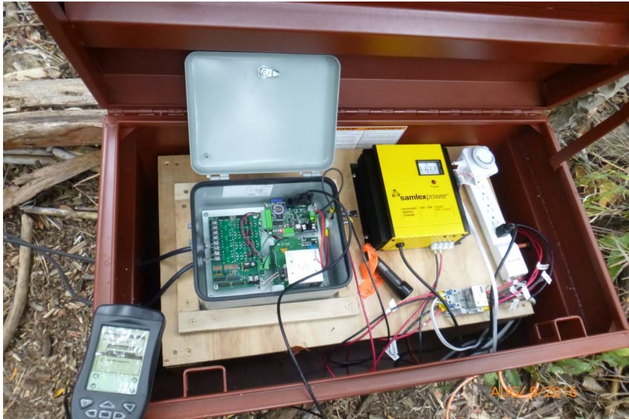
Figure 5. Picture of the surge protector, battery charger, relay, and PIT tag reader contained within a protective jobox at the AC-powered Ventura mainstem PIT tag array site. Two batteries are contained beneath the wooden board.
