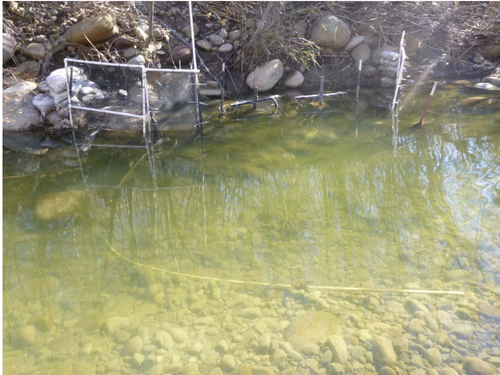
Figure 10. Picture of PVC pipe dislodged from earth anchor wire breakage during January 19, 2017 storm event. Shown from wide-angle (a) and close-up (b) perspectives.
